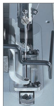
Position of the needle bar during sewing
